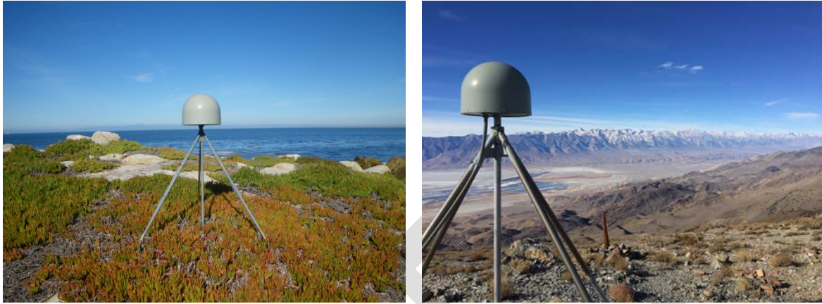
Figure 2. Left – UNAVCO station P231 at the Hopkins Marine Station in Monterey Bay is a SDBM (short drilled-braced monument) with stainless steel legs extending 1.75 meters and epoxied into bedrock. The station was installed by UNAVCO during the National Science Foundation-funded EarthScope project originally to measure earthquake and tectonic deformation along the San Andreas and San Gregorio faults. In addition, now the station is used by a variety of stakeholders for surveying, sea level analysis, tropospheric water vapor studies, soil moisture, coastal LiDAR surveys, and ionosphere electron count that can be used for tsunami early warning. Data is streamed from this site via direct Internet connection. Right – Station P466 Cerro Gordo in the Inyo Mountains is a DDBM (deep drilled-braced monument) with stainless steel legs extending 10m into bedrock that was installed to monitor the Owens Valley and Death Valley faults systems. Now it also serves as a critical station for water resource monitoring (reference Borsa, 2014 and others)
